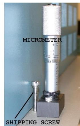
Tilt micrometer with shipping screw partially removed
