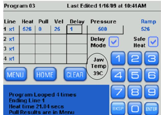
Figure 18. Jaw temperature.
