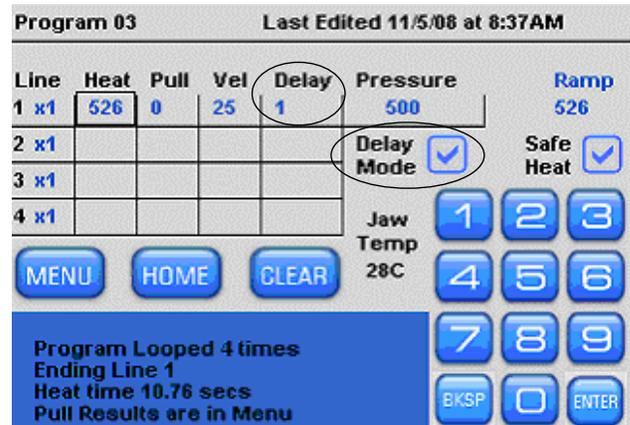
Figure 17. Delay mode of air-cooling.
