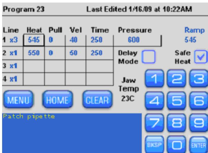
Figure 13. Two-line program with first line looped.
