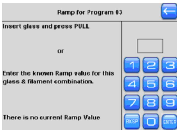
Figure 7. Ramp test.
