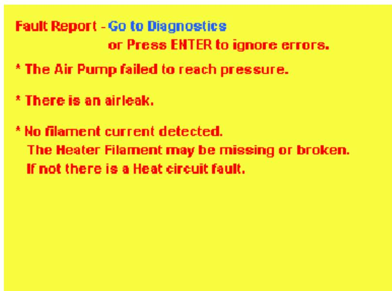
Figure 2. Startup fault report screen.
