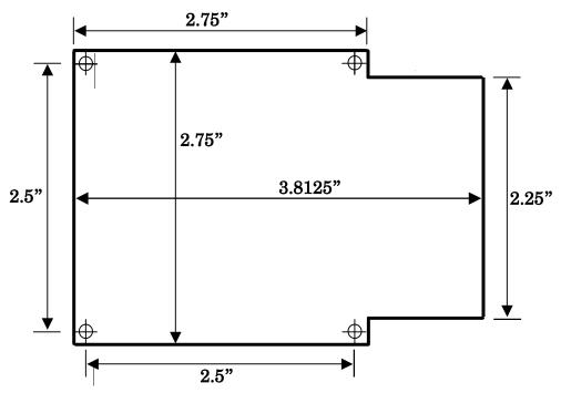
Figure 2-5. Manipulator base dimensions.
