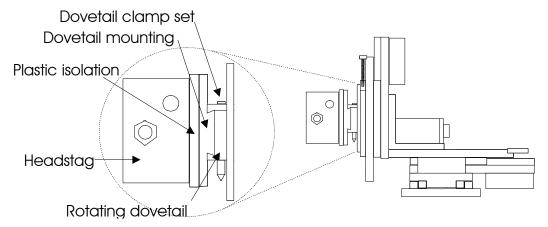
Figure 2-7. Mounting the headstage on the manipulator's Z-axis.
