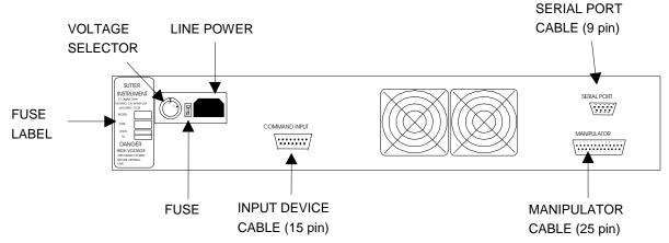
Figure 2-4. MP-285 controller rear connections.
