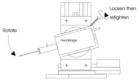
Figure 2-8. Adjusting the headstage angle.
