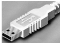
Figure 5-3 -- Host connector end of USB cable.
