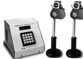
Dual SmartShutter (25-pin to two 9-pin split cable) configuration
