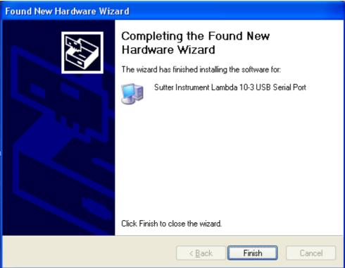
After installing the driver successfully open <Device Manager> and you will see the device shown in the Bus and Ports folder.
