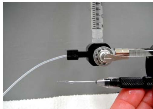
3. Replace the pipette and turn the selector back facing east. Then use the coarse dial on the injector or the 3cc syringe to fill the pipette.
