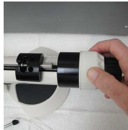
6. Fill a 3cc syringe with oil or water and make sure there are no air bubbles. Screw it onto the top port of the 3-way valve and position the selector east. Then turn the coarse dial of the injector clockwise six complete turns to advance the plunger and introduce oil/water into the 3-way valve.
