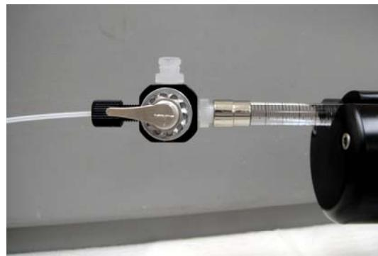
4. Return the selector facing west, remove the 3cc syringe (optional) and continue injecting/transferring.
