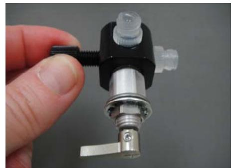
5. Insert tubing through rear connector and install the ferrule. **First** attach the 3-way connector to the Hamilton syringe and **then** attach rear connector to the three-way valve.
