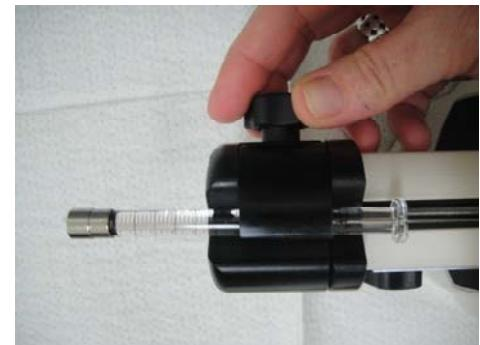
2. Turn the coarse dial on injector (counter clockwise) to draw back the plunger retaining block and install the oil or water filled Hamilton syringe onto XenoWorks Analog Injector. Make sure the front and back ends of the syringe are not sitting within the groove of the black clamp. Tighten the rear screw that holds the end of the metal plunger in place. Then tighten the knob and clamp onto the glass body of the Hamilton syringe.
