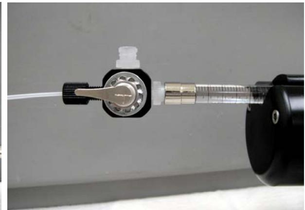
10. Turn the selector west to begin using the injector. You may now remove (optional) the 3cc filling syringe.
