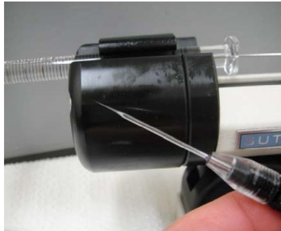
8. Turn the clear plastic tip of the pipette holder  $\frac{1}{2}$  turn to loosen the seal, allowing you to insert your pipette. Push the pipette all the way into the holder (the o-rings might offer some resistance) until it goes no further. The holder is designed to accept 1mm outer diameter glass. If you are using glass with a 1.2mm or 1.5mm OD, contact Sutter Instrument to purchase a custom holder to accept the size of your glass.
