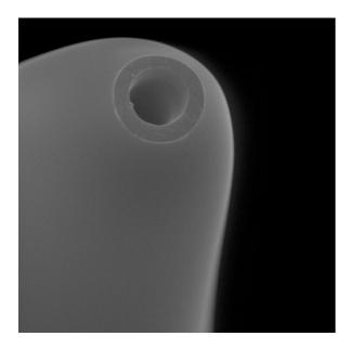
Fabricating Nano Electrospray Ionization Emitters from Fused Silica Capillary Tubing on the P-2000/F Micropipette Puller
