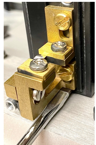
STEP 4. Slide jaw down 3mm and pry up to adjust.
