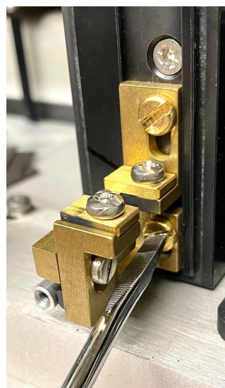
STEP 3. Loosen bottom brass screw.
