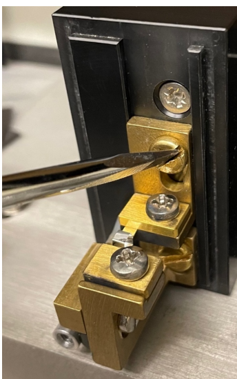
STEP 1. Loosen top brass screw.
