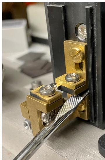
STEP 2. Slide down 3mm and pry up to adjust.
